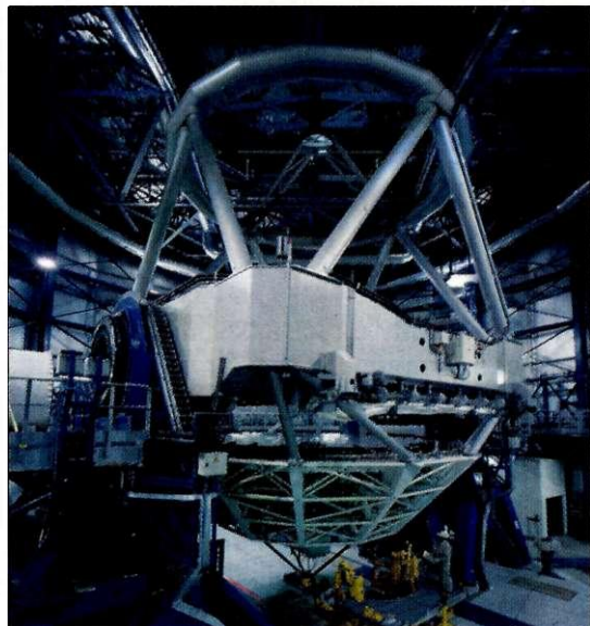
The first of the VLT's 8.2 m mirrors.
