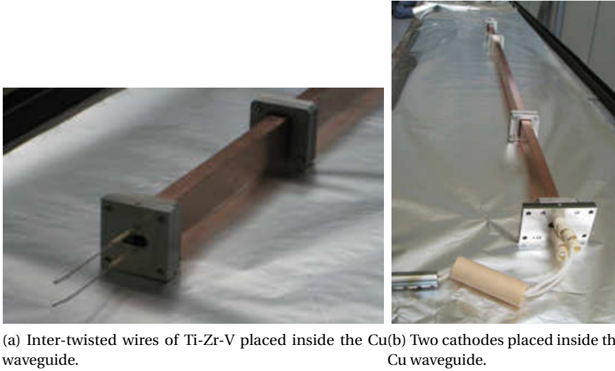
Figure 4.13: Preparation of the Cu waveguide for the NEG coating.
