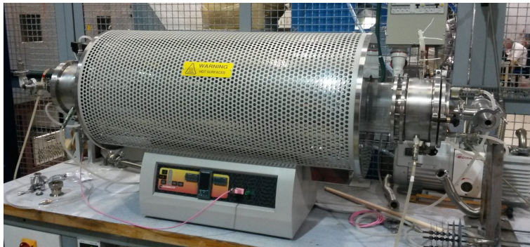
Figure 6.7: Furnace used for the heat treatment of the cable stack. Argon was flowing in the oven during the heat treatment. Two stacks could be treated at once.
