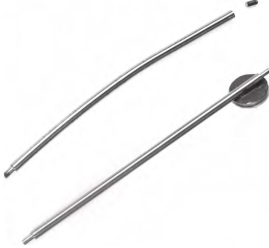
Figure 4.9: Beryllium rods for the neutrino target installed at the SPS designed to be impacted by 1 \times 10^{13} protons with a momentum of 300 \text{ GeV } c^{-1} . The device on top was accidentally hit by an off-axis beam, leading to permanent bending and failure of the rod [58].
