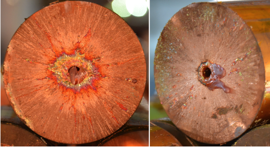
Figure 4.8: Front face (left) and back face (right) of a copper cylinder after an impact of 2.16 \times 10^{13} protons with a momentum of 440 \text{ GeV } c^{-1} [50].
