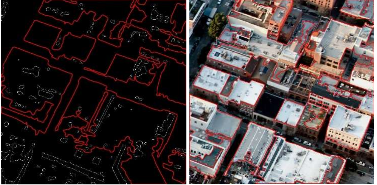
Figure 31 represents the images introduced in Figure 13 The two original images used to demonstrate BIM's stitching process after Figure 14 Illustrated BIM process used for image stitching's steps 1, 2, 3, 4, 5 and 6.a, Shape contouring using The-Chin algorithm. The right image presents shape contouring directly applied on the original image for comparison.
