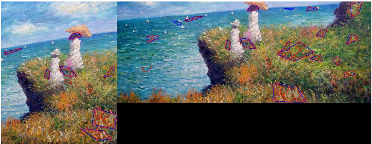
Figure 52 Amount of image successfully stitched depending on perspective intensity, with a sample of image at the maximum noise tolerance. In red, key points selected as described in Shape contouring blobs comparison chapter and in blue key points selected as described in Convex hull blobs comparison chapter.
