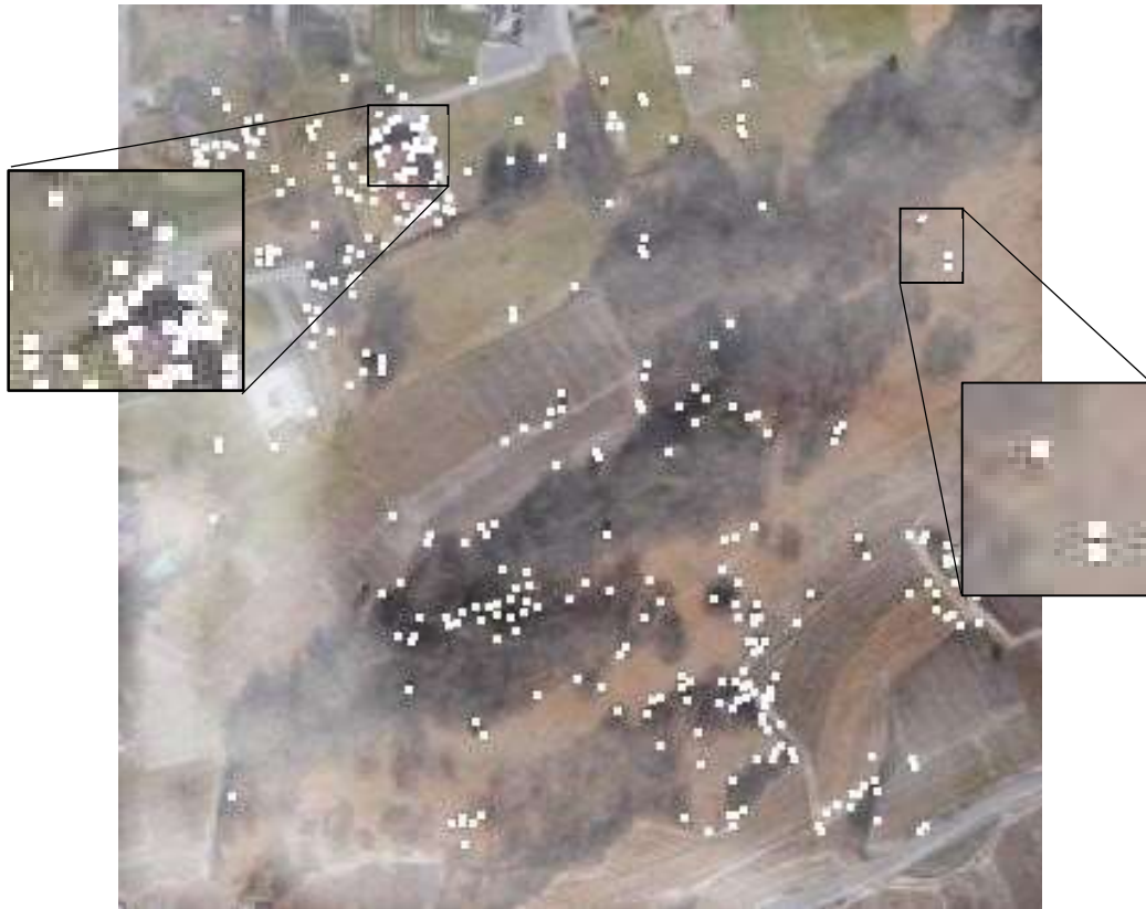
Figure 10 Shows a FREAK implementation for features detection, using the Accord.net framework. The image shows although it is less visible than in Figure 6 Shows a Harris implementation for features detection, using the Accord.net framework. The image shows that the techniques holds on camera lenses' partial obstruction and detects no points in the clouded area that the techniques holds on camera lenses' partial obstruction it moreover still detects few points in the clouded area.
