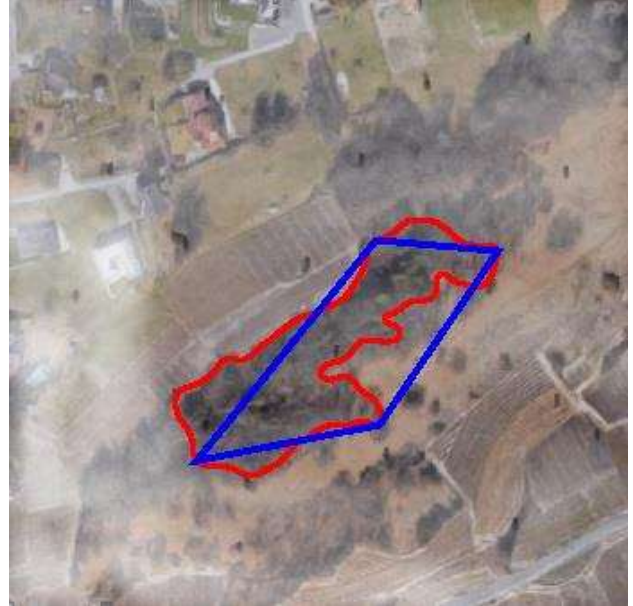
Figure 12 echoes with Figure 4, presenting BIM-s blob detection after the pre-processing steps presented in 3.6 Blurred Images Matching process. This specific feature detection detects 5 points, which is sufficient for a homography, as in the case of this image all the points are usable.
