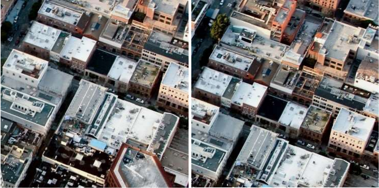
Figure 20 Images presented in Figure 13 The two original images used to demonstrate BIM's stitching process and Figure 17 Images presented in Figure 13 The two original images used to demonstrate BIM's stitching process after Histogram normalization. after brightness correction, here the images presents an average brightness of 113.
