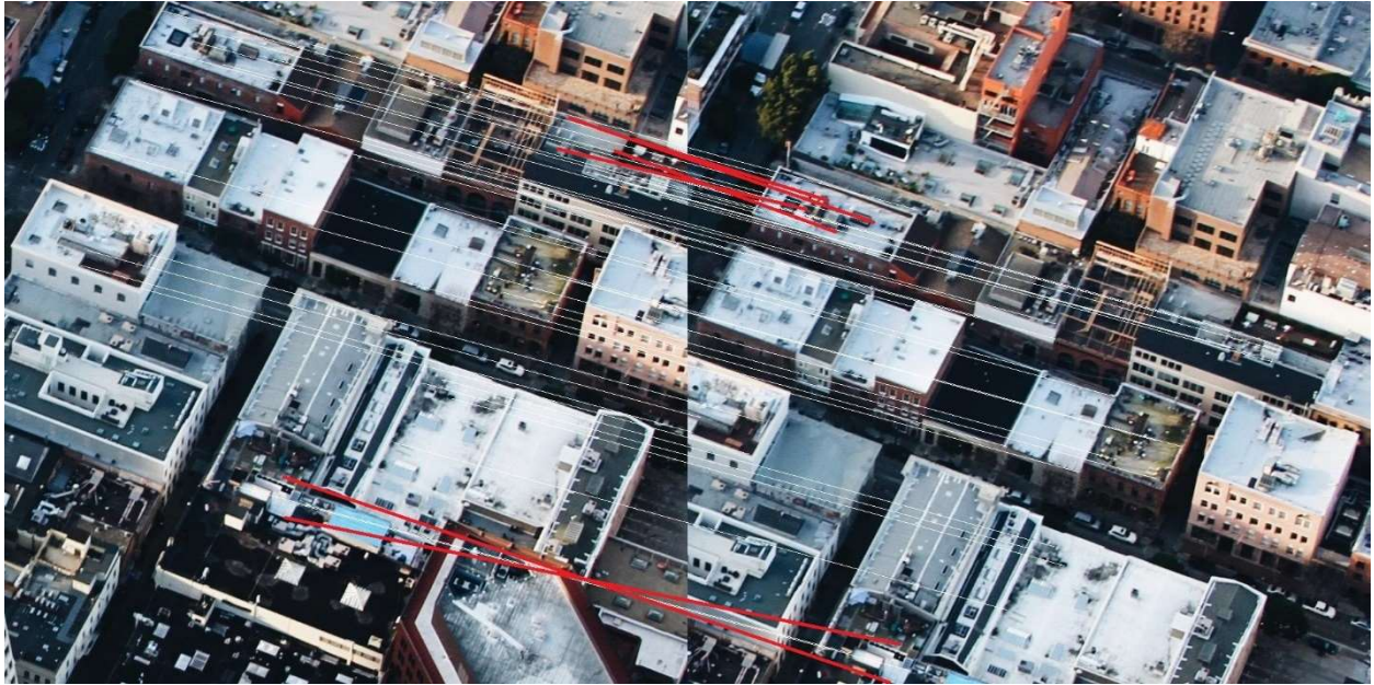
Figure 34 represents points correlated between the pair of image introduced in 3.6.2 and at step 7 of Figure 14 Illustrated BIM process used for image stitching. Outliners are highlighted in red; those outliners perturb greatly the homography if not filtered out.
