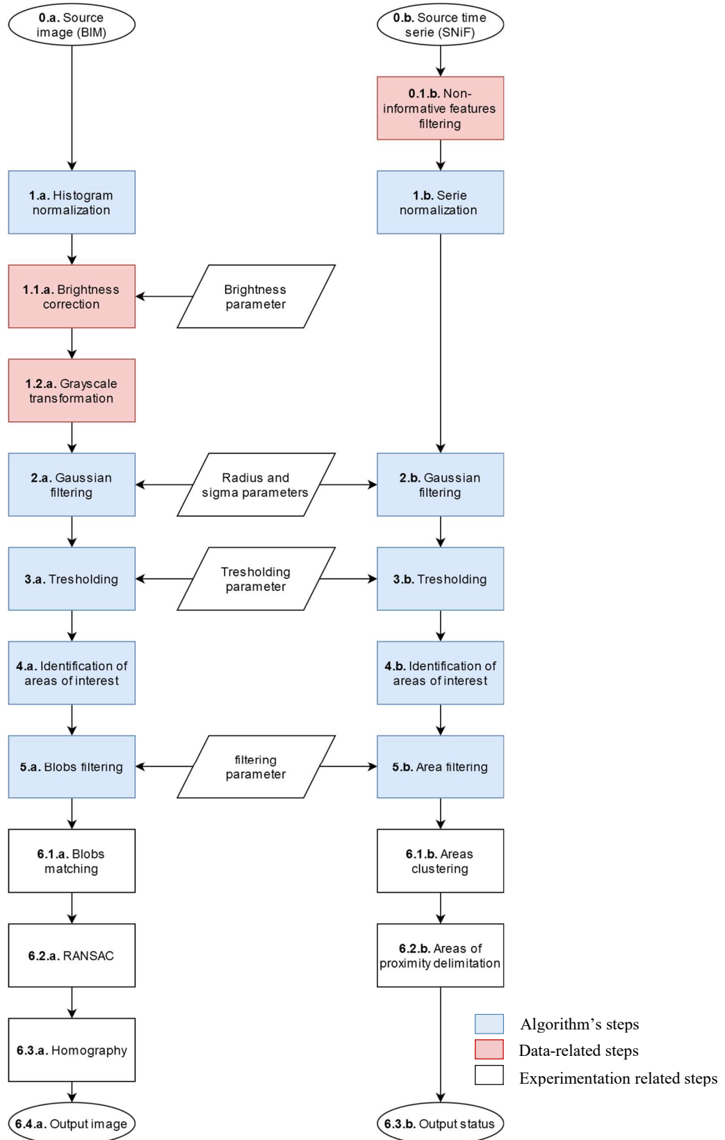
Figure 88 BIM and SNiF process comparison with similar steps (blue) steps depending on the data source (red) and step relative to the experimentation (white).
