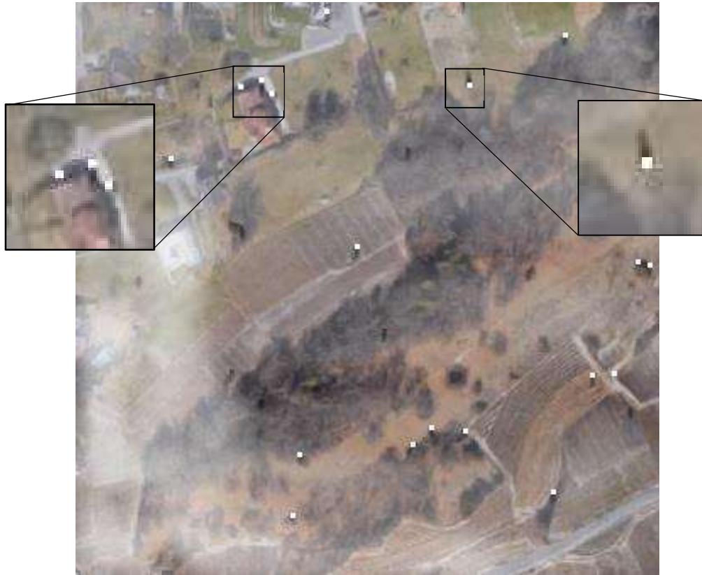
Figure 6 Shows a Harris implementation for features detection, using the Accord.net framework. The image shows that the techniques holds on camera lenses' partial obstruction and detects no points in the clouded area.
