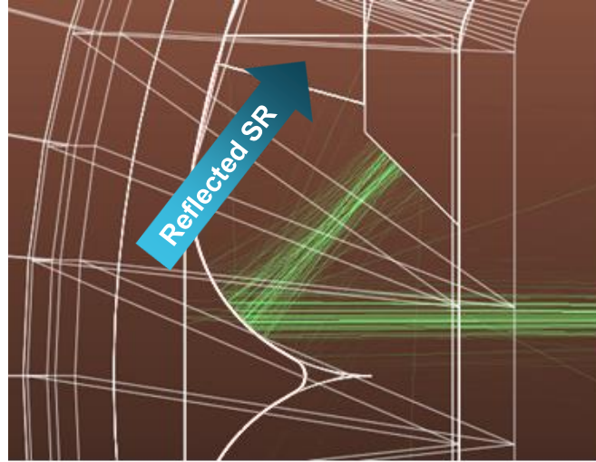
FIGURE 4.8: Detail of a ray tracing simulation showing the SR impacting on the BS sharp reflector with the 50 TeV proton beam vertically misaligned 2 mm. In this case, the SR is not reflected as intended by design.
