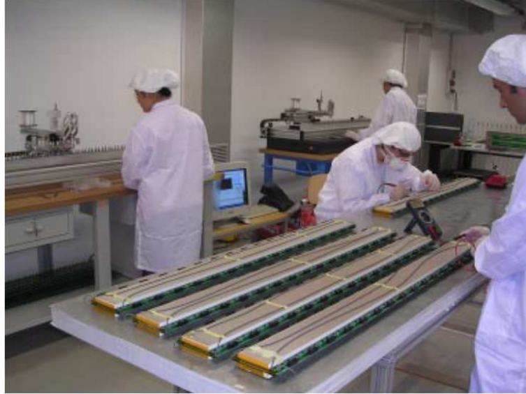
Figure 2.19: MRPCs production at Bologna-INFN laboratories.
