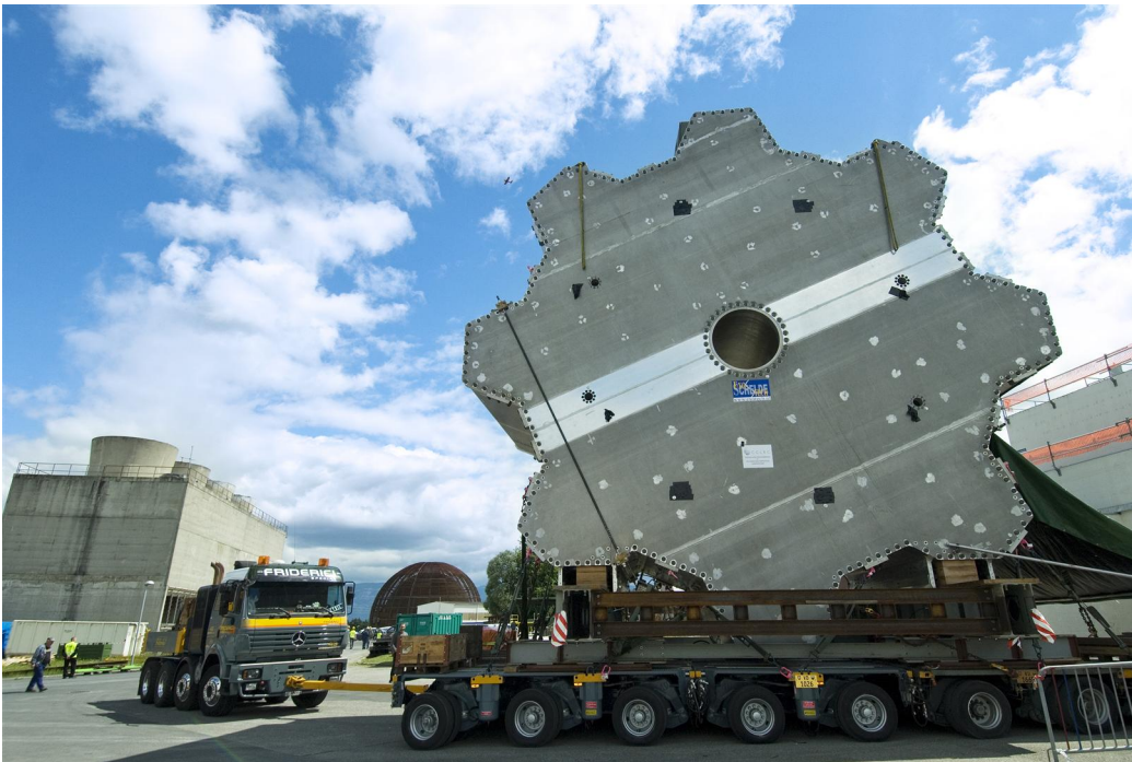
FIGURE 2.12: A picture of one of the two ATLAS end-cap toroids. Ref. [68].
