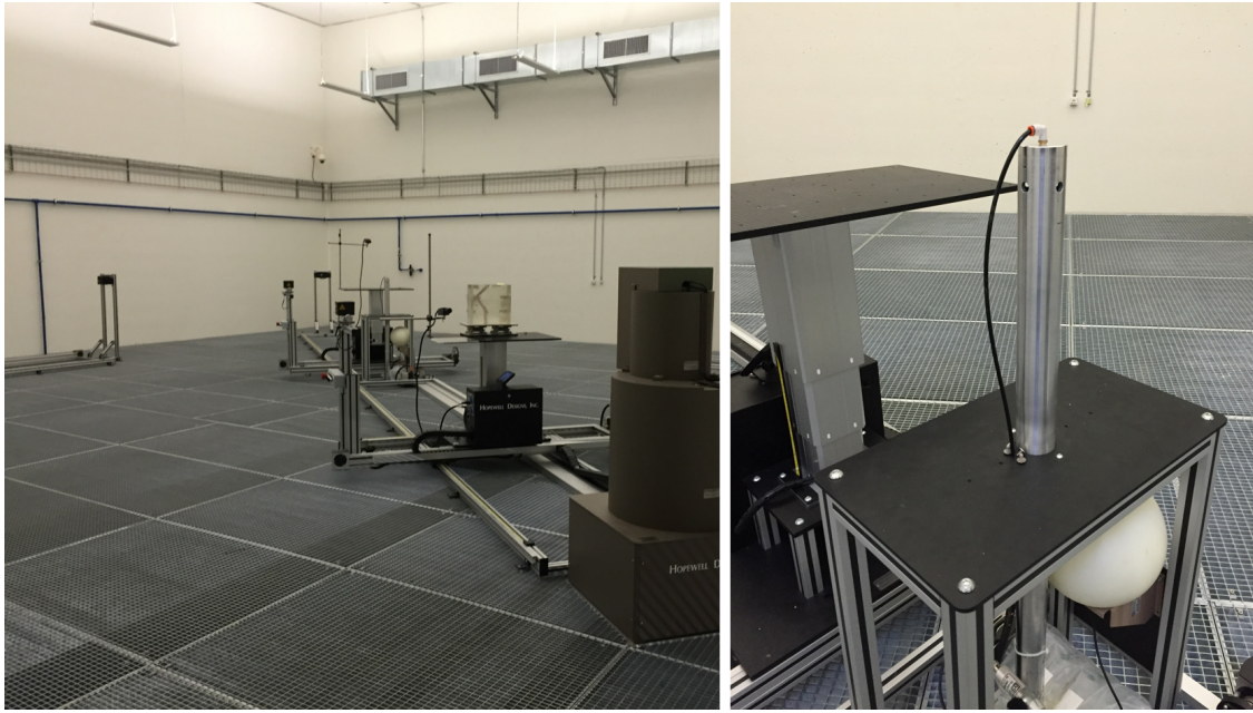
Figure 4.14: Am-Be irradiation room.
