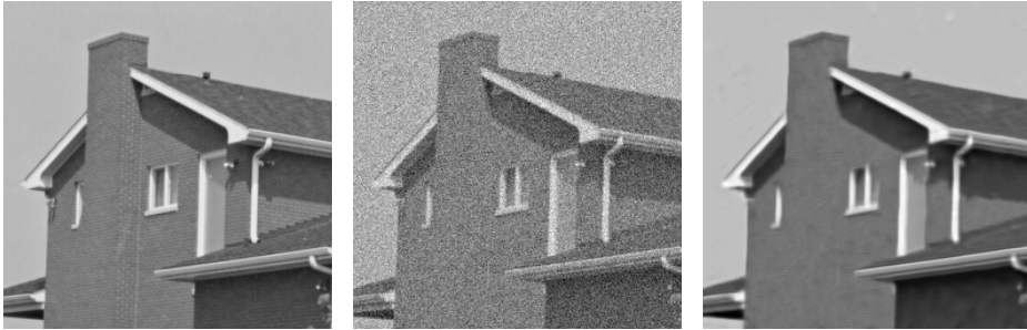
Figure 4.8: Left: Noiseless “house” image. Center: Image with additive Gaussian noise applied ( \sigma = 25 , PSNR = 20.19 dB). Right: Image denoised with EEM for BSC (PSNR = 32.32 dB).
