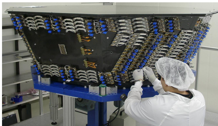
Figure 3.9: Picture of the TRD during assembly, showing the inverted octagonal pyramid shape. Credit: Ref. [ AmsWebsite ]
