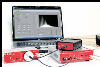
Set-up for SiPM testing & characterization
