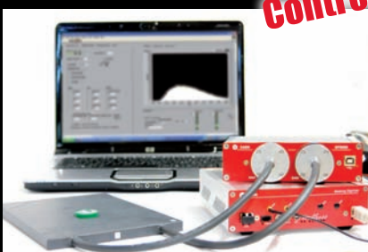
Set-up for detecting cosmic rays and \beta particles
