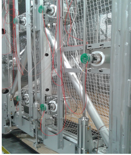
Figure 14: Part of the ICARUS T600 module with the installed PMTs.
