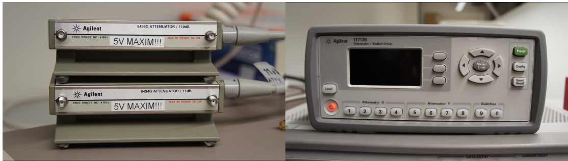
FIGURE 7.17: Agilent 11713B 8496G 8494G variable attenuator used for linearity measurements
