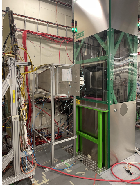
Figure 6: Setup of the ME0 stack in front of the source at the GIF++.
