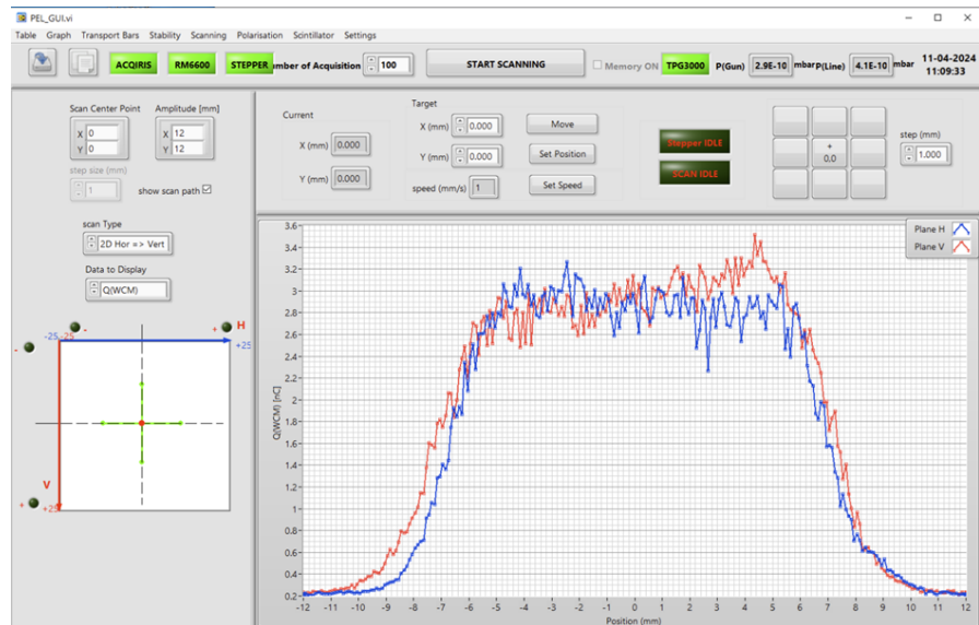
FIGURE 4.8: LabVIEW interface for centering the beam on the photocathode. Example for cathode #217 with the OPO at 266 nm, after proper alignment.
