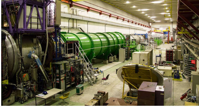
Figure 2.14: A picture of the downstream part of the NA62 detector. The RICH green vessel is clearly visible; on the left there is the gray tank of the LKr calorimeter; between the LKr and the RICH, the CHOD is partially visible; the blue MNP33 magnet of the STRAW spectrometer can be spotted on the right.
