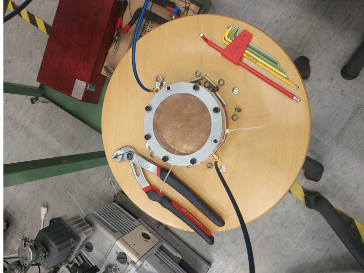
Figure 5: The set-up that we used in the lab, consisting of a copper plate on top of the dielectric resonator, connected to the VNA
