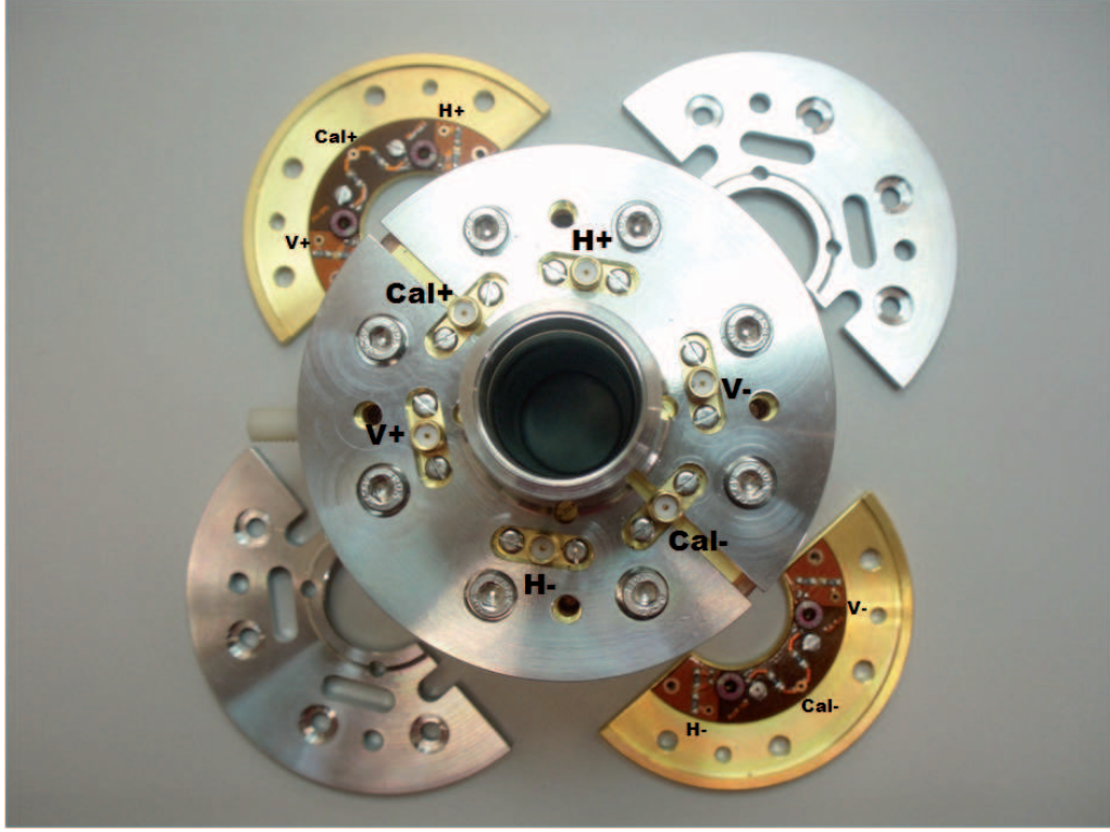
Figure 3.4: Top view of the BPS prototype to show the SMA output ports and calibration input ports, labeled with their names; and the PCBs outside with the toroidal transformers.
