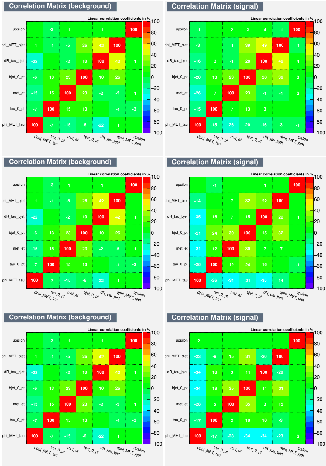
FIGURE 6.4: Correlation matrix of BDT input variables for the backgrounds (left plots) and signal (right plots), the H^+ mass ranges, 130-160 GeV (top), 160-180 GeV (middle), 200-400 GeV (bottom). Here: \text{upsilon} = Y ; \text{dphi\_MET\_bjet} = \Delta\phi_{b\text{-jet}, E_T^{\text{miss}}} ; \text{dR\_tau\_bjet} = \Delta R_{b\text{-jet}, \tau} ; \text{bjet\_0\_pt} = p_T ; \text{met\_et} = E_T^{\text{miss}} ; \text{tau\_0\_pt} = p_T^\tau and \text{dphi\_MET\_tau} = \Delta\phi_{\tau, E_T^{\text{miss}}} .
