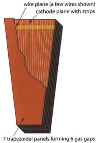
Figure 2-16: A CSC consists of seven panels forming six gas gaps. The radial cathode strips and azimuthal anode wires are shown (only a few anode wires are drawn).
