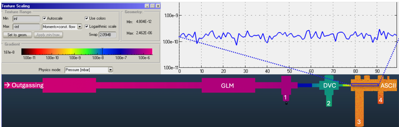
Figure 11: Molflow simulation of ASCII setup for H_2 . Outgassing rate: 250 \frac{mbar \cdot l}{s \cdot cm^2} . For pump rates of pumps 1-4 see above. Final pressure in ASCII chamber: 2 \cdot 10^{-10} mbar
