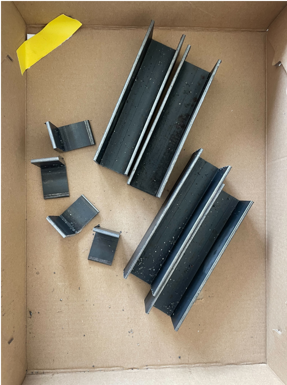
(a) Channel and angle piece of horizontal lead screw setup
