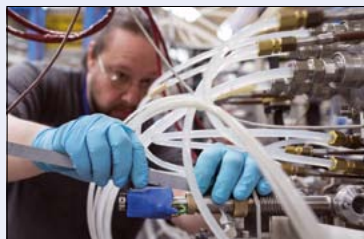
Every so often the source of the lead ions has to be replaced. A small sliver of solid isotopically pure ^{208}\text{Pb} is placed in a ceramic crucible that sits in an “oven” casing at the end of a metal rod. The metal is heated to around 800^\circ\text{C} and ionized to become plasma. Ions are then extracted from the plasma and accelerated.
