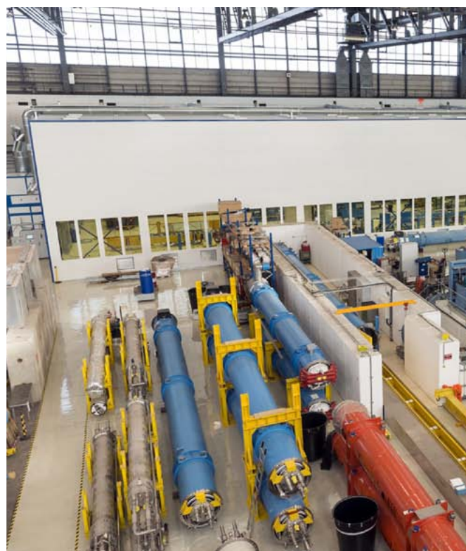
A view of the Large Magnet Facility in Building 180. To the left are spare cryomagnets, with the welding press on the right and the mock-up of a magnet string for training purposes just behind.
