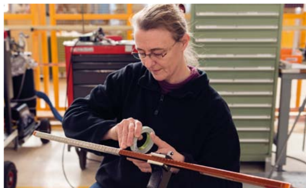
Applying electrical insulation to a busbar to equip a mock-up.
