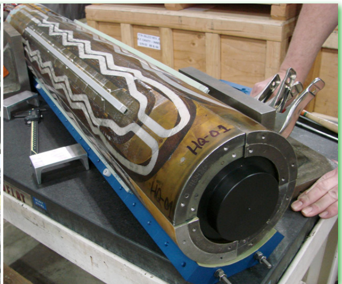
The 1 m long quadrupole developed by the US-LARP collaboration. During recent tests, the quadrupole successfully reached 13 T of magnetic field.
