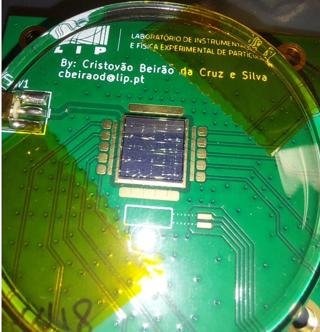
Figure 9: Wirebonded LGAD. Not every pixel has its own readout. Some of them are wire bonded to the same readout pad on the PCB.
