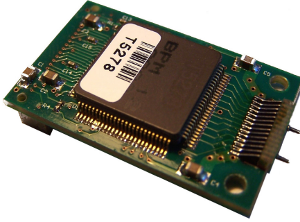
Figure 3.6: Photograph of a TX-plugin ( 34 \times 21 \text{ mm}^2 ) with the prominent BPM12 ASIC and the VCSEL laser array for transmission to the front-end electronics, picture taken from [52].
