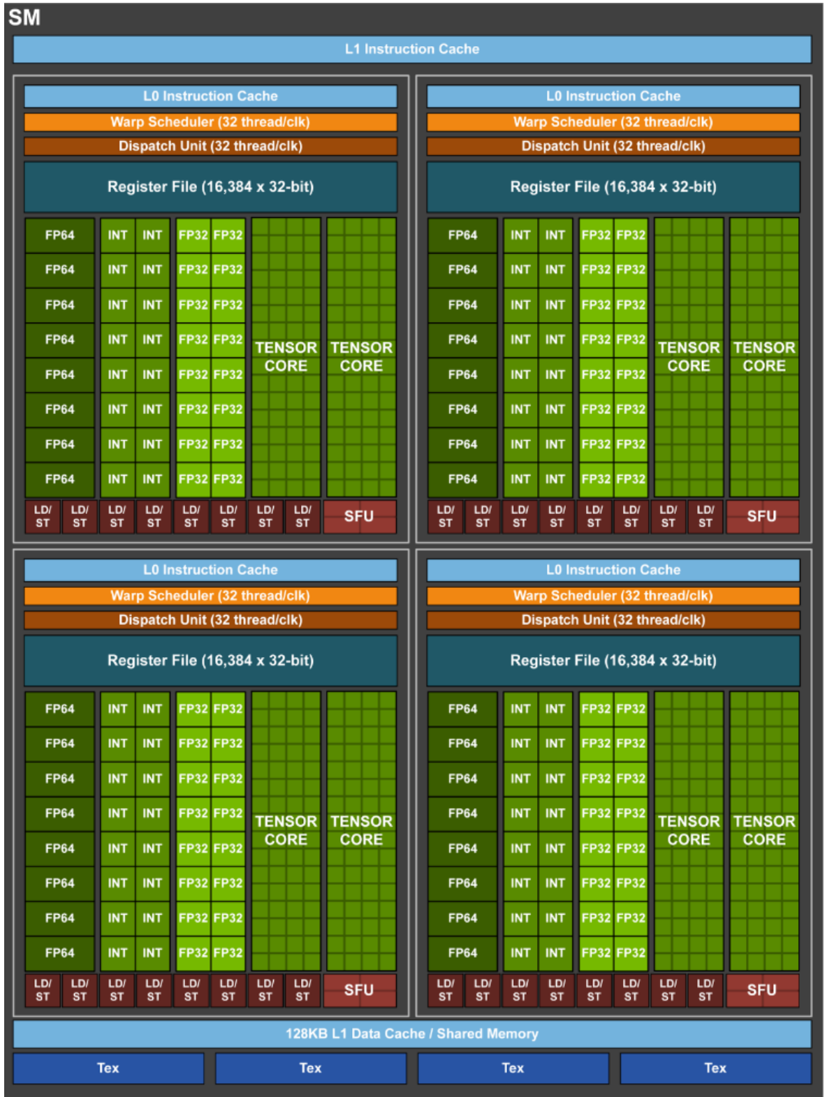
Figure 13: V100 Streaming Multiprocessor containing several different computing cores, load/store units and caches [28].
