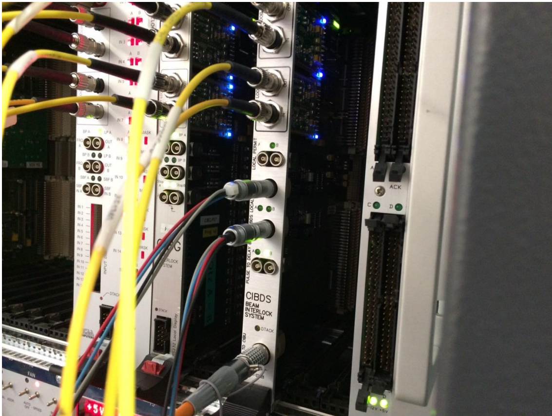
Figure 8.3: Photograph of the CIBDS prototype in the testing rack.
