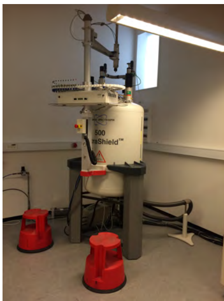
FIGURE 7.1: Bruker UltraShield Avance spectrometer at University of Copenhagen, 500 MHz (11.74 T).
