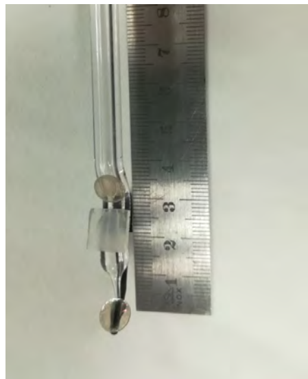
FIGURE 8.14: Glass capillary system front view, as the radioactive beam sees it.
