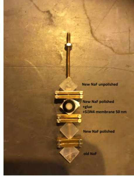
FIGURE 8.2: Sample holder arrangement of the second and third experimental campaigns.
