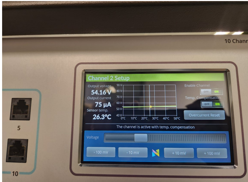
Figure B.5: Voltage supply for the detector with temperature compensation.
