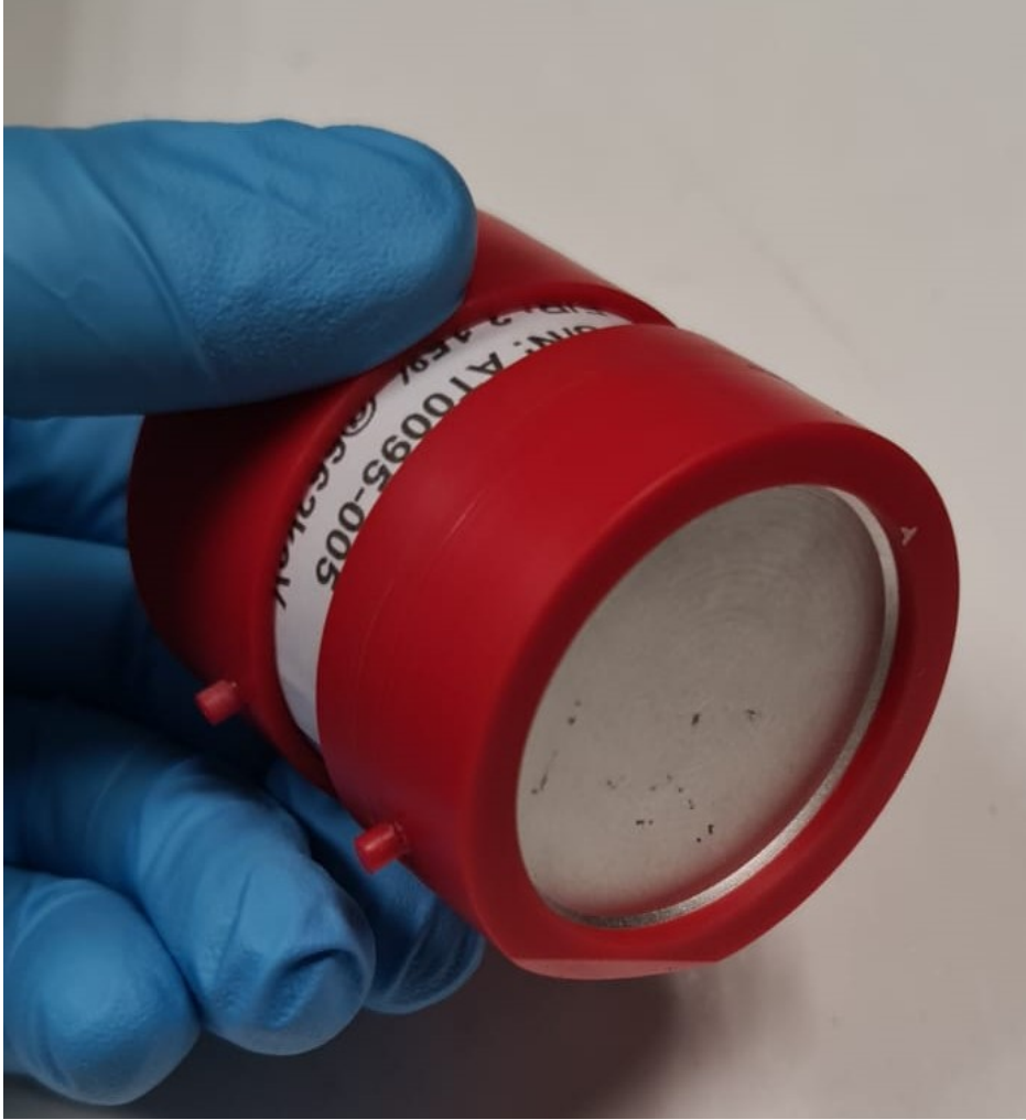
Figure A.3: Two red plastic objects got stuck on the \text{LaBr}_3 (Ce) scintillator crystal. Also, the side for the gamma photon penetration is visible.
