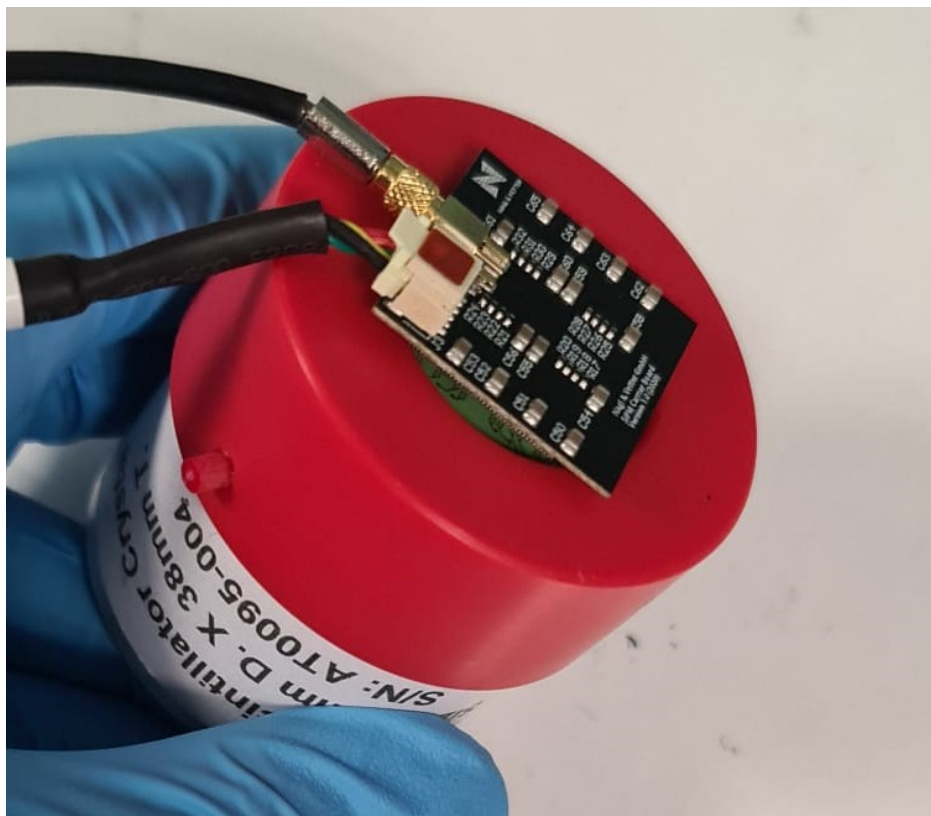
Figure A.5: Fully constructed detector connected to the U5310A digitizer and to a voltage supply.
