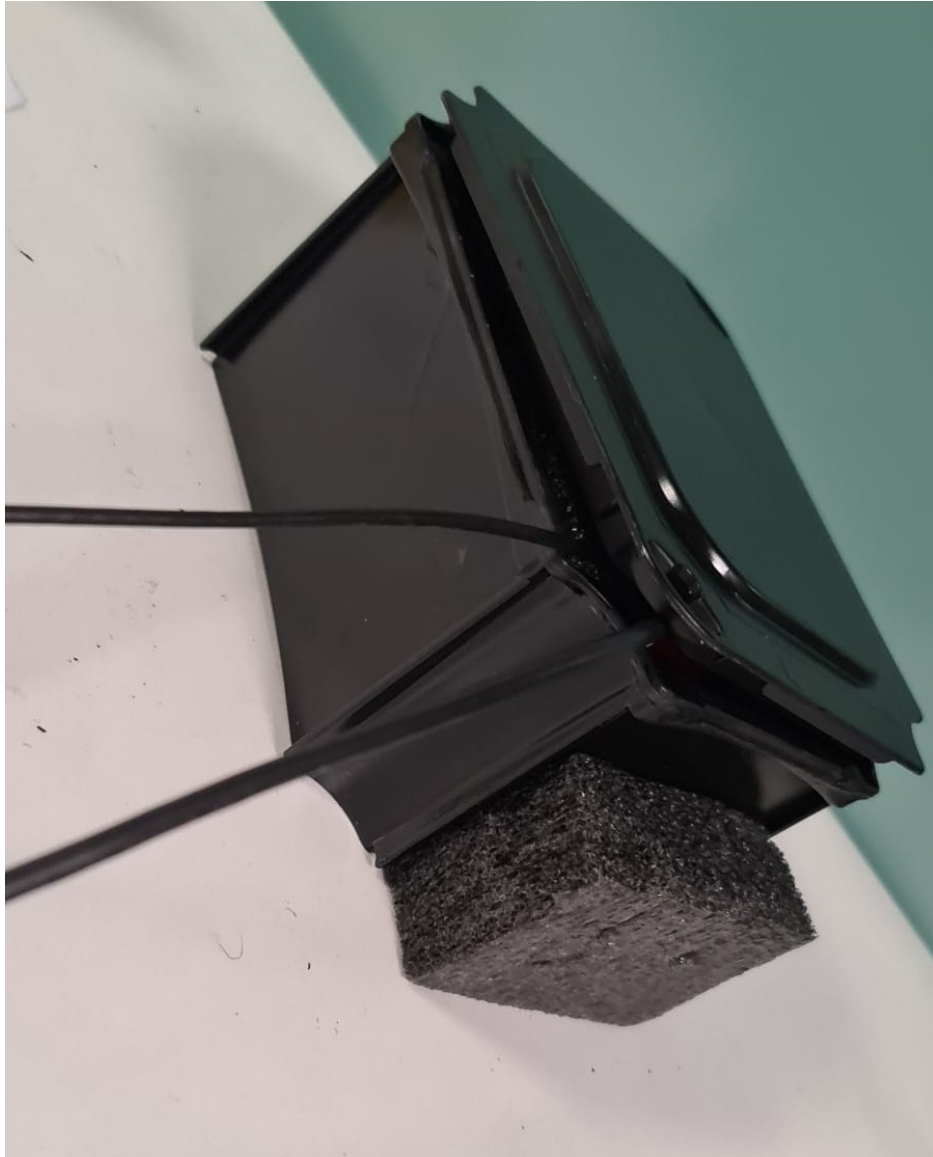
Figure B.3: Closed black box with detector and cobalt 60 source inside; the cables are going out.
