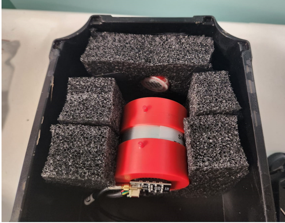
Figure B.2: Opened black box with detector and cobalt 60 source inside.
