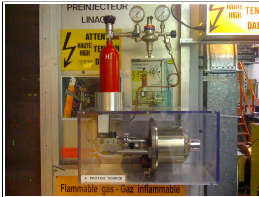
Figure 2.4: The LHC proton source.
