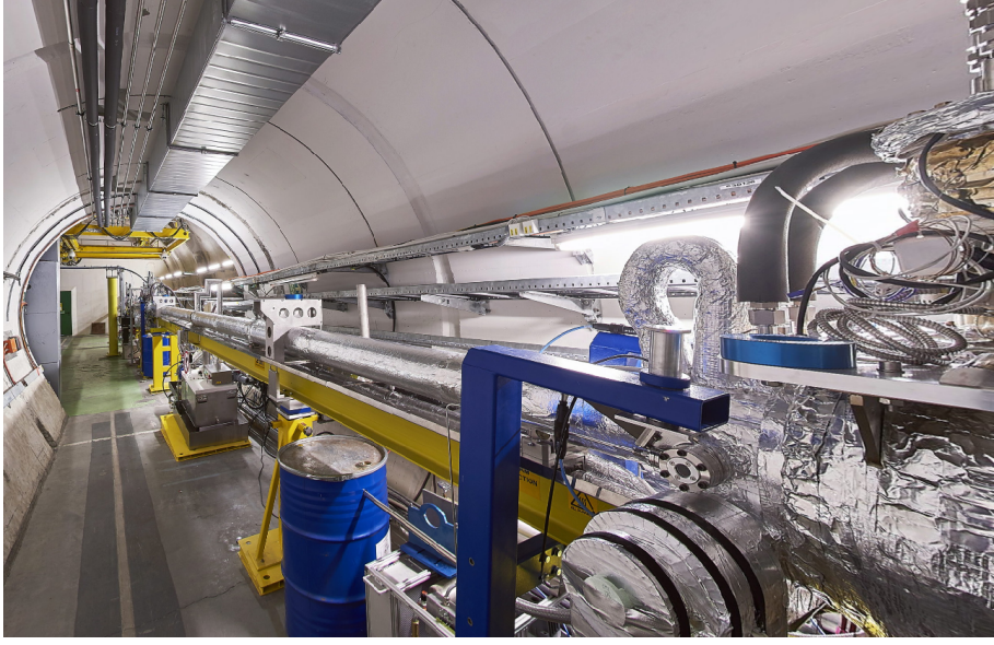
Figure 2.4: Picture of the 10 m long vapor source in the AWAKE facility [Photo: Maximilien Brice, CERN].
