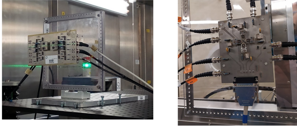
Fig. 4.14: Photo of Board 1 (left) and Board 2 (right) placed inside the irradiation room, in front of the beamline.
