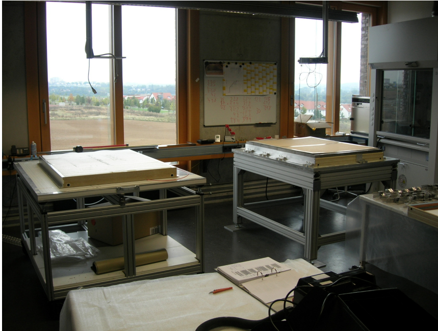
Figure B.1: The table for the frame assembly (right) and the vacuum table for the gluing of the back panel (left). The aluminum plates are especially designed and machined with very high precision of a maximum deviation of less than 0.1 mm.
