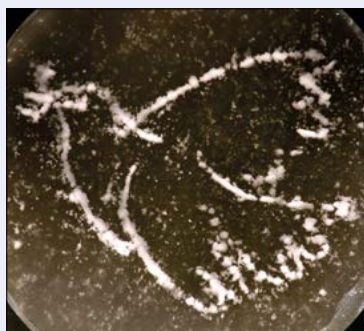
Ultrasonic waves were used to push a collection of microparticles into the shape of Picasso's peace dove. (Image credit: K Melde/MPI for Intelligent Systems.)
