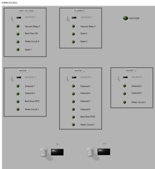
Figure 5.30: UI: Interlock Status of EBTS
