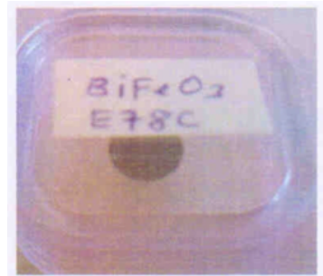
Figure 6.4: BFO pellet before ^{111}\text{In} implantation.
