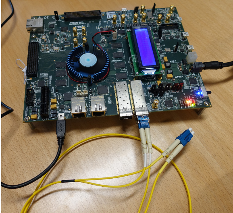
Figure 87: ArriaV in loopback mode
