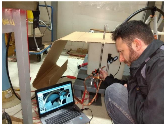
Fig. 64. a (upper left). b (upper right). c (bottom left): The set-up for recording breakdowns in DC
