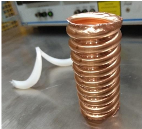
Fig. 81. The actual spirally corrugated OC and the helical spacer
