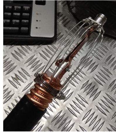
Fig. 73. Specially made connector for connecting with the VNA cable
