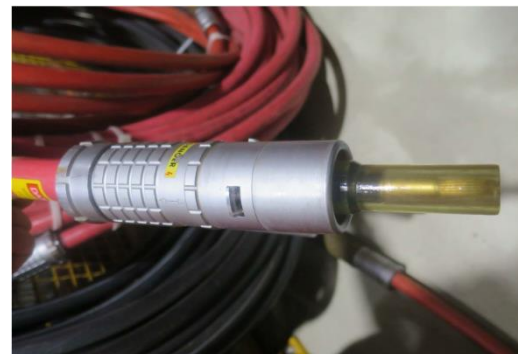
Fig. 21. LEMO HT50 connector, in use for system voltages up to 40kV [19]
