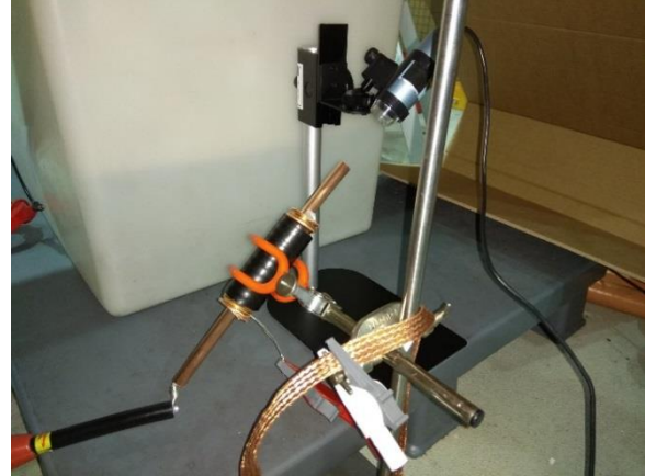
Fig. 64. a (upper left). b (upper right). c (bottom left): The set-up for recording breakdowns in DC
