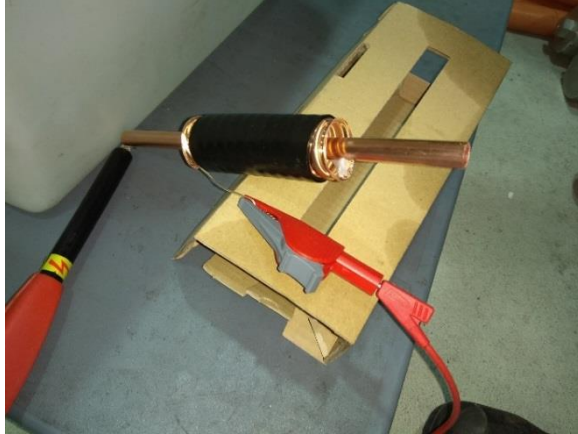
Fig. 64. a (upper left). b (upper right). c (bottom left): The set-up for recording breakdowns in DC
