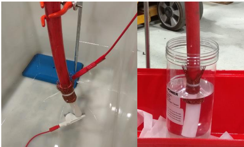
Fig. 71. Cable ends in oil
