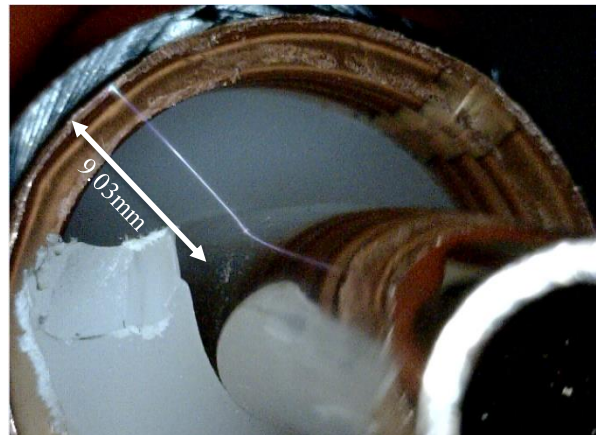
Fig. 65. An electric arc during a breakdown in air
