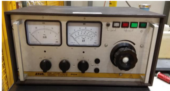
Fig. 35. BAUR PGK 110 operating unit
