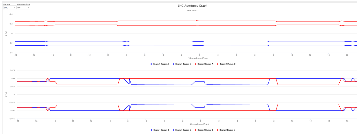
Figure 2.34: Aperture graph around IP4, where the Superconducting RF Cavities are installed. One cannot even notice that RF cavities are installed at this location.
