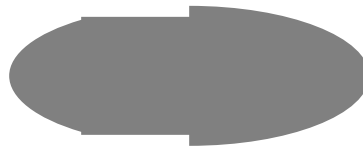
Figure 2.31: Aperture shape with the jaws opened in parking position (maximum) at \pm 29mm [4]. Data gathered from drawing [28].
