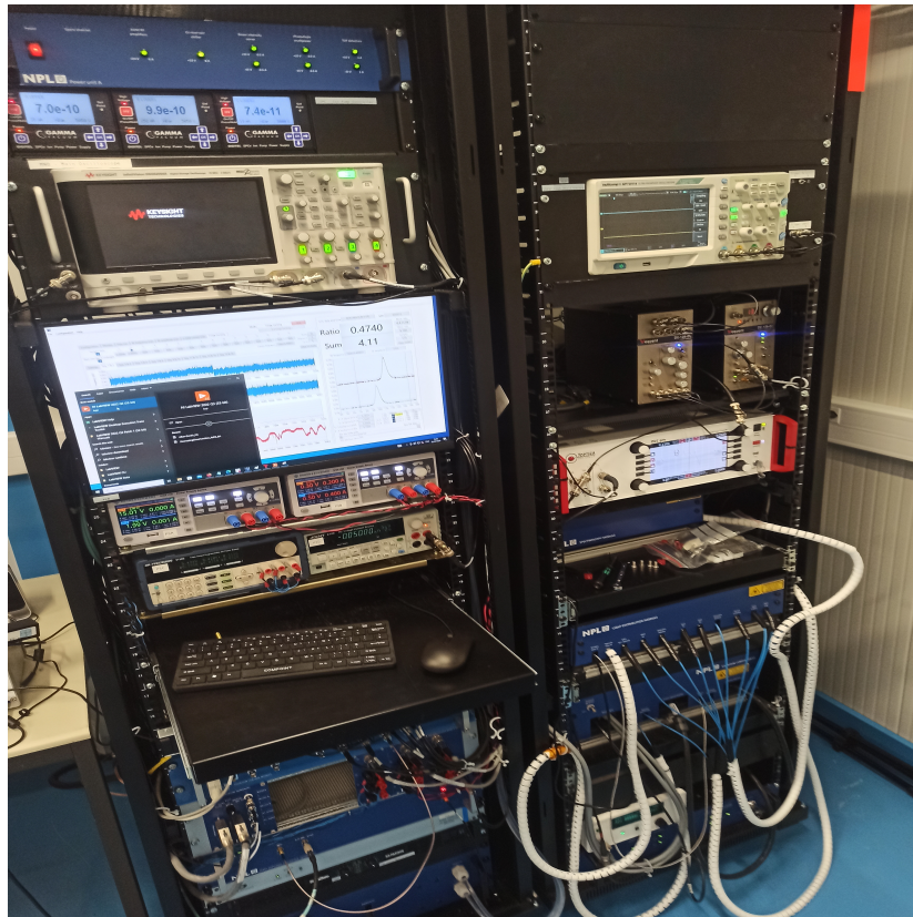
Fig. 4. The computer that controls the caesium fountain. At the top, there are three indicators displaying pressures: 7.0 \times 10^{-10} , 9.9 \times 10^{-10} , and 7.4 \times 10^{-11} , these correspond to vacuum levels of the caesium fountain.
