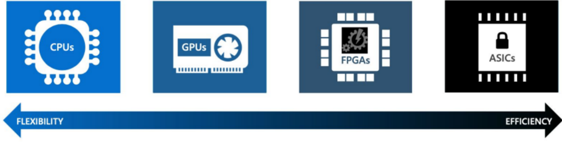
Figure 2.6. Comparison of different computing architectures: flexibility vs. efficiency [28].
