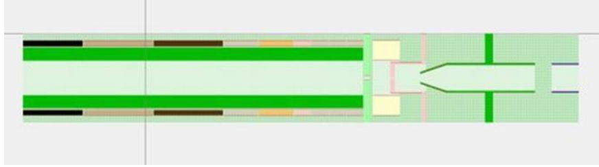
FIGURE 6; YZ Cross section for electrodes extraction. The right hand side shows the electrodes of the extraction system.
