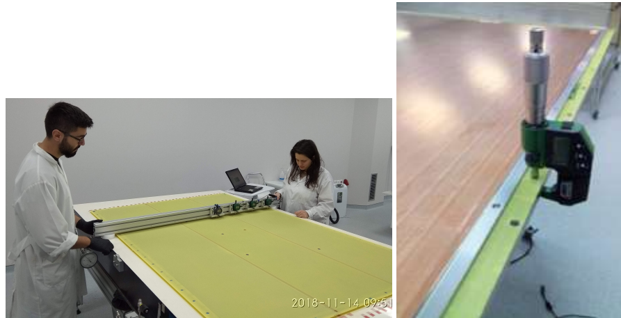
FIGURE 3.18: Measurement of thickness and planarity with limbo tool (left) and perimetrical thickness measurement with digital micrometer (right).
