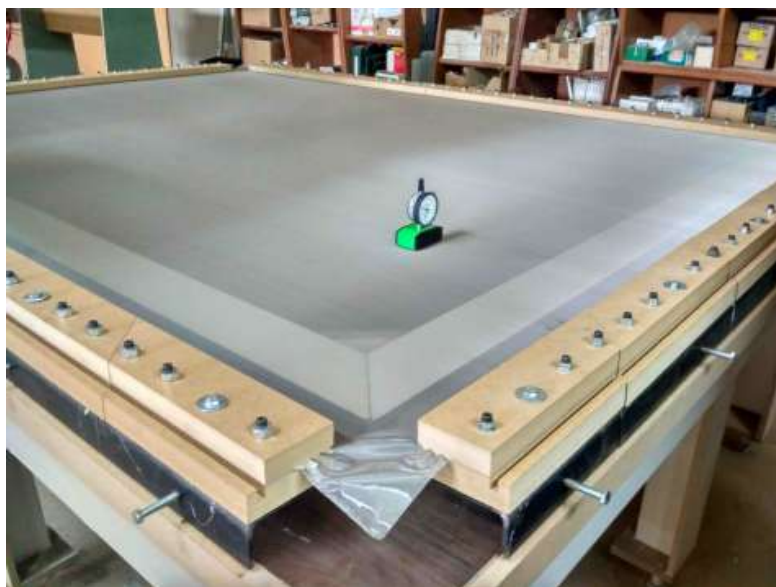
FIGURE 3.15: Mesh stretched on custom made table and tension measurement
