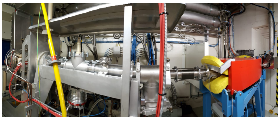
Figure 1.2: A picture of the CERN-MEDICIS experimental setup, where medical radioisotopes are extracted from a target and filtered using mass separation. Image taken from [13].
