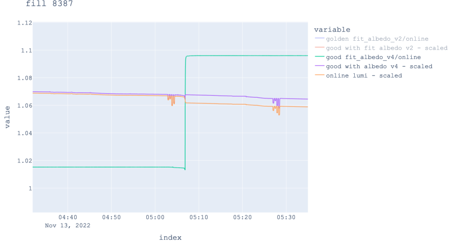
Figure 6: Online and offline (reprocessed) luminosity data from the BCM1F in 2022. Notice the sudden drop in the online data after 05:00. The purple line is the reprocessed luminosity
