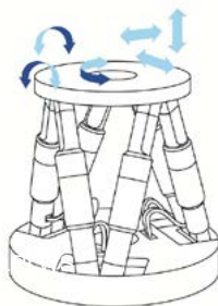
Fig 2: Basic design: In parallel-kinematic systems, all actuators act directly on the same platform. (image: PI)
