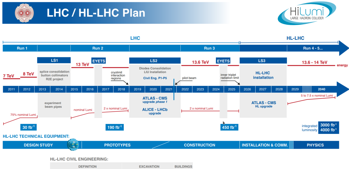
Figure 1.12: Schedule of interleaved periods of data collection and long shutdowns with a projection for the instantaneous and integrated luminosities and collision energies at the LHC [21].
