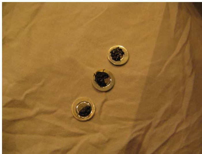
Fig. 2.27: Filters clogged using epoxy glue on different surface portion of the filters
