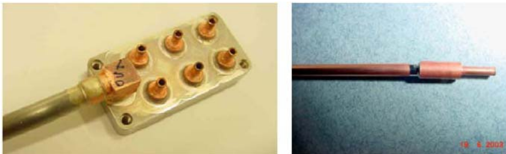
Fig. 2.2: The cooling collector and the Phynox tube with the Cu fitting
