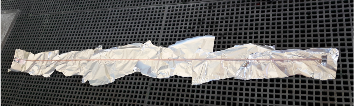
Figure 7.5. 4mm diameter, 2 meters length, NEG coated chamber.
