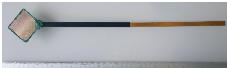
Figure 5.7. Platelets after copper PVD coating, before electroforming.
