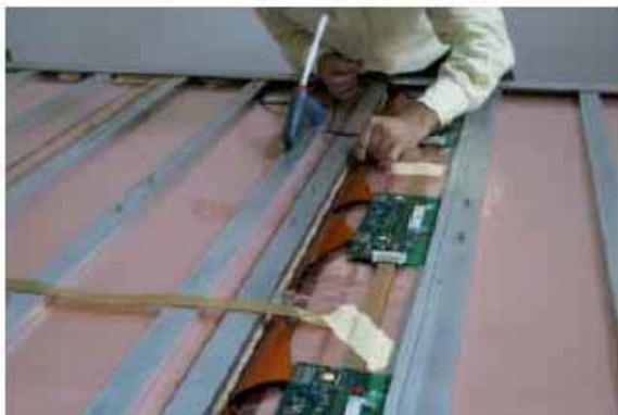
Figure 28 A technician assembling a RPC
